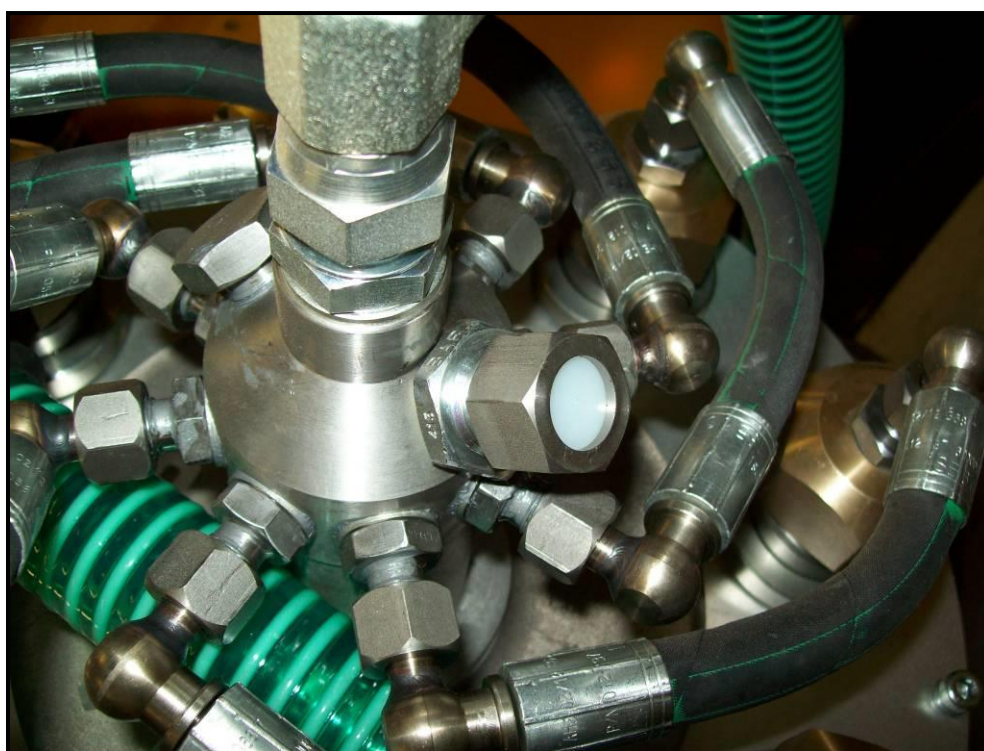
Fig. 6.2 Burst disc holder showing 'white' burst disc
